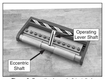
Figure 3. Operating lever shaft installed.
